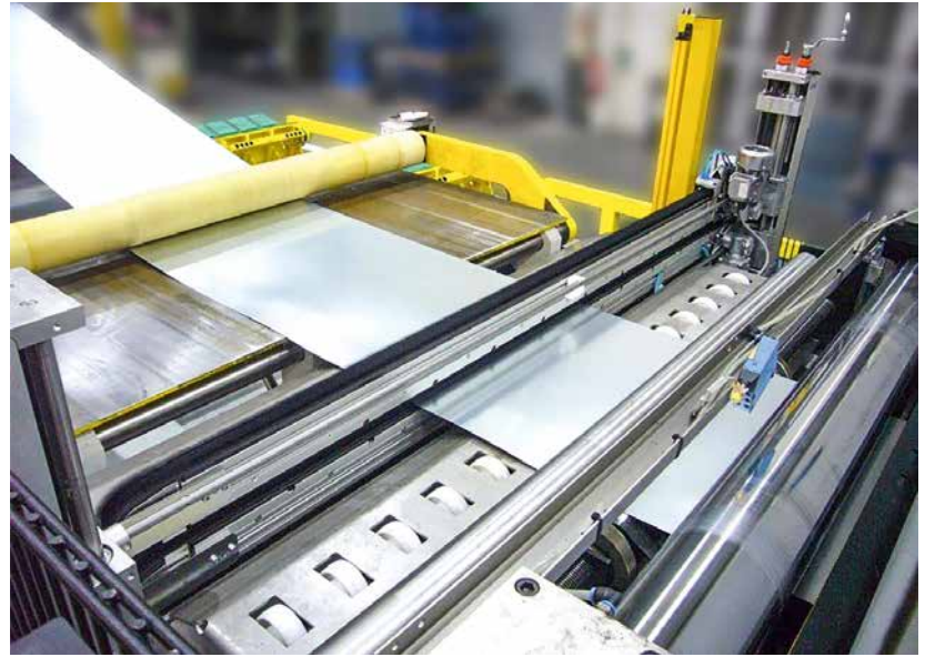
A Combi Sword Brush cleaning a steel strip from above and below.
