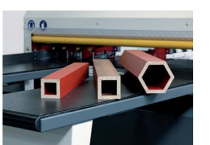
Because boards are cut to size and mitre cuts are performed simultaneously on only one machine, there is no need for handling from one saw to the next. This significantly reduces the risk of errors and damage.
